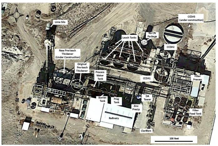
Figure 21.1 Shafter Processing Facility
