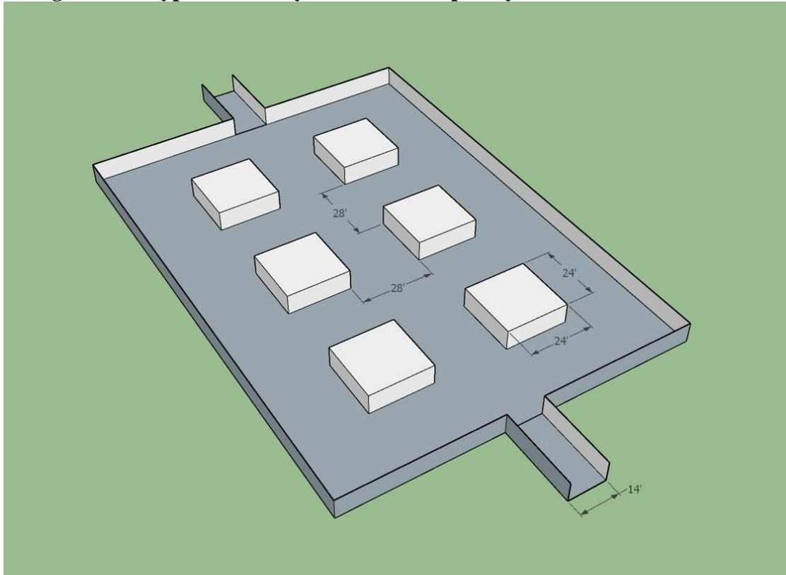
Once the primary extraction sequence in each work area is complete, secondary extraction would include combinations of: slashing pockets of back material, benching floor areas that meet cutoff, slashing of ribs, and partial pillar recovery. Once pillar recovery starts the stope areas would only be accessible with remote controlled equipment.
